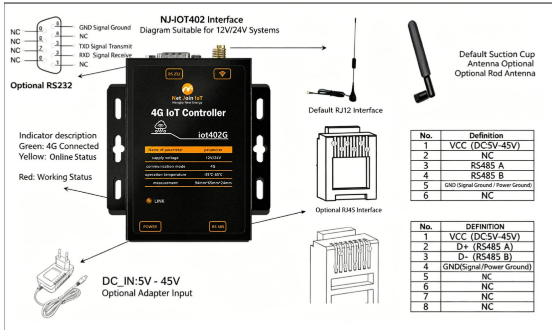
NJ-iot402WE Wiring Diagram
